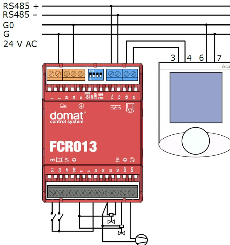
**Power supply G and G0 terminals are internally connected with G and G0 terminals on the input/output terminals block (lower row).**
