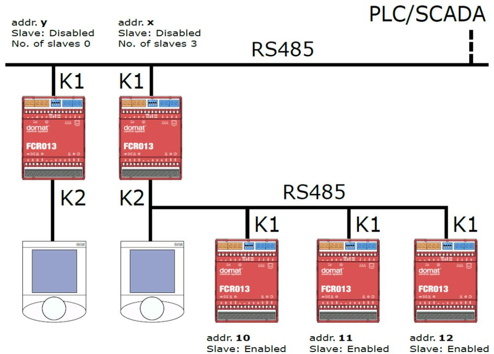
In this connection, controllers with addresses x, 10, 11, and 12 are in one zone and all of them are controlled by one room unit. The controller addressed x is a master. Outputs of controllers addressed 10, 11, and 12 are controlled by the same signals as the master controller addressed x.
